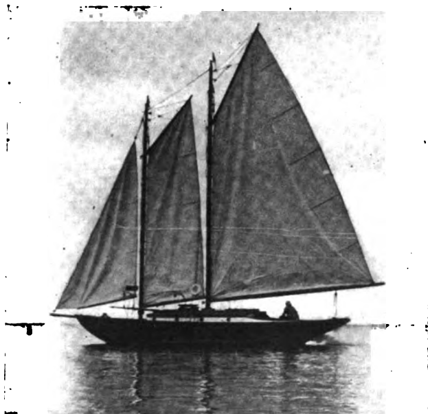
Phydoro, Aux. Schooner, 43 x 30 x 11 ft. 6 in. x 4 ft. 6 in. Power 2-cyl. 15 H.P. Keystone Engine, H. Lawrence Hess, Jr., Owner. Designed by Messrs. Bowes & Mower and Built by John Kirk, Toms River, N. J.
